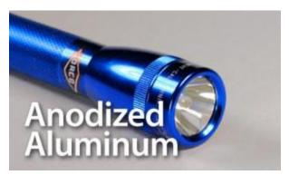
Aluminum must be anodized in order for dye to adhere to the surface. Anodizing is the process where a thin layer of oxidized aluminum is produced. This is achieved by placing the aluminum in an electrolytic bath consisting of an acid solution. An electric current is passed through the solution using the aluminum as the anode (positively charged) and a negatively charged cathode. This causes a layer of aluminum oxide to develop on the surface of the aluminum. This layer
